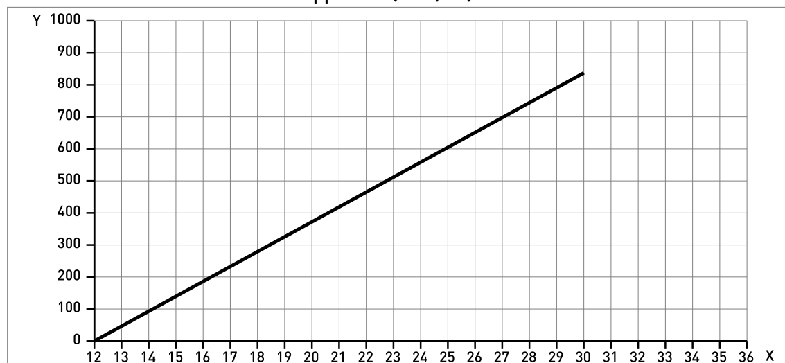
Figure 2-9: Minimum power supply voltage for an output of 21.5 mA at the terminals (Non-Ex and Hazardous Location approval (Ex i / IS))
