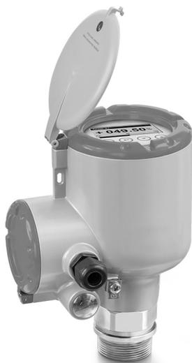
The small beam angle and negligible dead zone of this 80 GHz FMCW radar level transmitter makes it the premium choice for liquids in small and narrow tanks with internal obstructions like agitators or heating coils, as well as tanks with long nozzles. It can even measure through tank roofs made of non-conductive material (e.g. plastic, fiberglass or glass). The flush-mounted PEEK Lens antenna (no tank intrusion) is insensitive to deposit.
