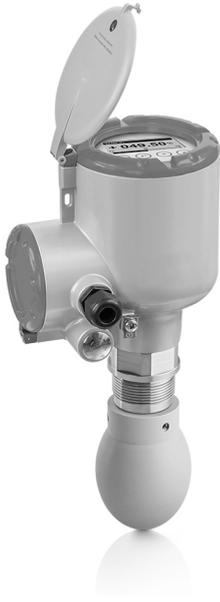
Designed for basic liquid applications, this market entry 24 GHz 2-wire FMCW radar transmitter provides accurate readings even in fast moving processes, in closed tanks or in the open air like rivers or dams. Its proven PP Drop antenna is insensitive to condensation.
