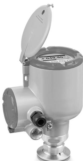
This 80 GHz FMCW radar transmitter for hygienic liquid applications in the pharmaceutical, food and beverage industries is CIP-SIP suitable and offers a large choice of hygienic process connections: Tri-Clamp®, Tuchenhausen VARIVENT®, SMS, DIN 11851, DIN 11864-1 Form A, NEUMO BioControl®.
