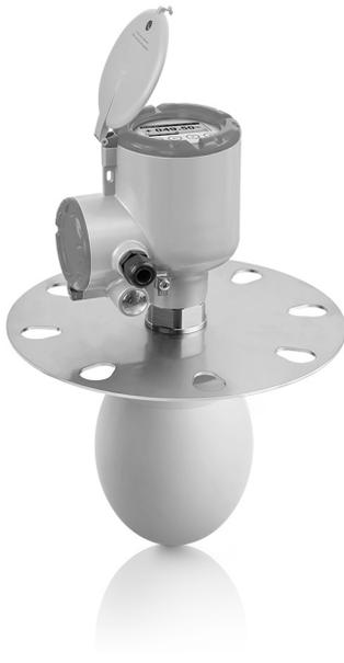
By combining high signal dynamics and FMCW radar technology, this market-entry 24 GHz radar device measures accurately and reliably the level of solids like stone, plastic granulates or coffee beans. No need for expensive antenna aiming kits or purging systems; the proven Drop antenna design minimizes scaling and is not affected by the angle of repose.
