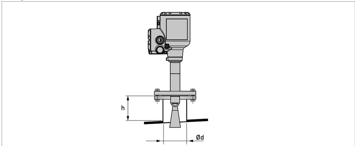
Figure 3-6: Flange connections
