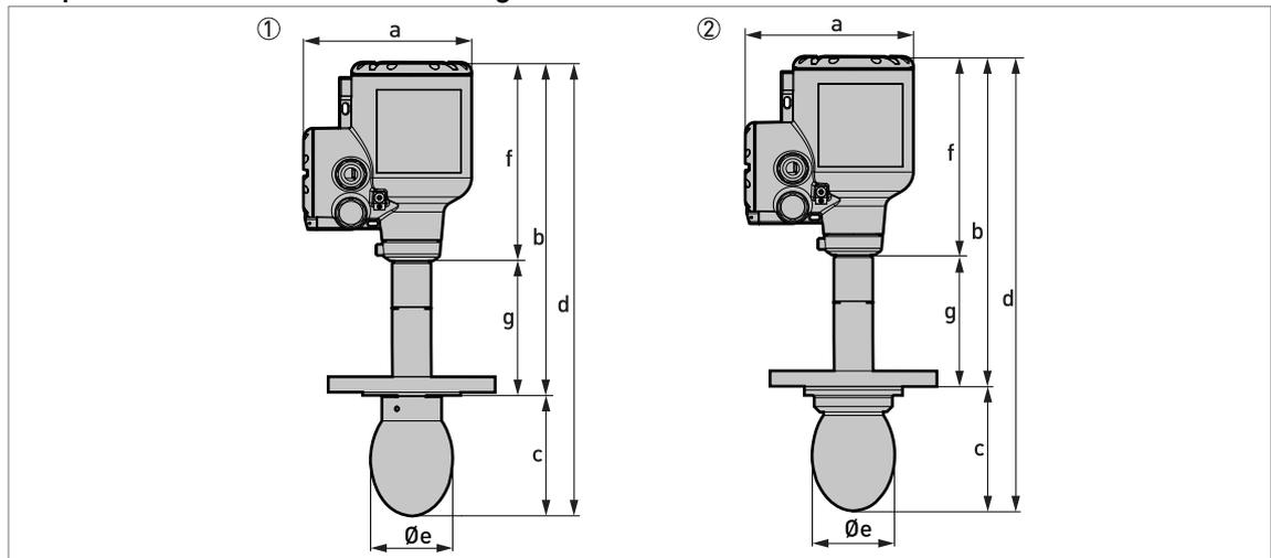
Figure 2-13: Drop antennas with standard flange connections
