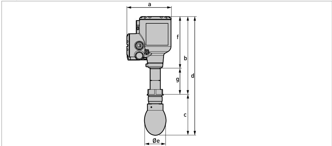
Figure 2-12: Drop antennas with threaded connections
