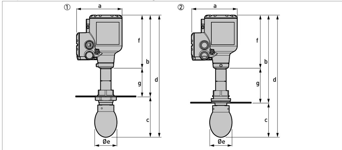
Figure 2-14: Drop antennas with low-pressure flange connections
