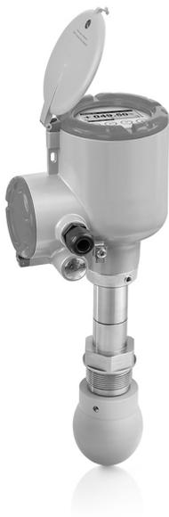
This 24 GHz FMCW radar level transmitter is designed for liquids in harsh environment like tanks with agitators containing corrosives or in non-Ex applications with extremely high process temperatures, like molten salt in solar plants (+700°C / +1292°F). For toxic and dangerous products, the use of a Metaglas® second sealing barrier is recommended.
