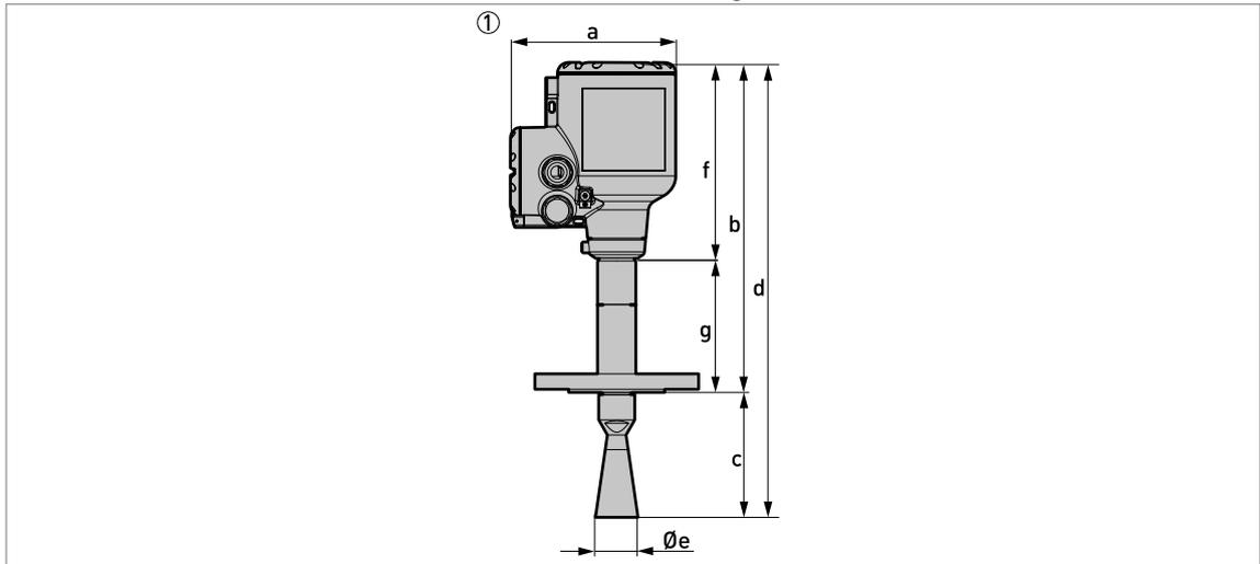
Figure 2-10: Metallic Horn antennas with standard flange connections
