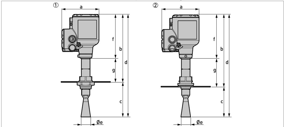
Figure 2-11: Metallic Horn antennas with low-pressure flange connections
