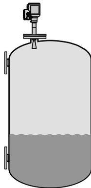
The level transmitter can measure the level of a wide range of liquid products on a large variety of installations within the stated pressure and temperature range. It does not require any calibration: it is only necessary to do a short configuration procedure.
