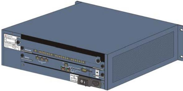
Use the metal ejector levers to pull off the blank panel.
