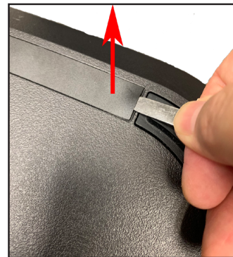
Figure 7. PC Sheets Removal
